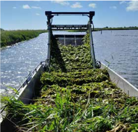
A water plant cutting vessel. Each vessel has a set of cutting knives attached to a conveyor belt, which cut the plants about a foot above the riverbed. The harvested plants are usually placed in low heaps on the bankside or taken to make compost. © Broads Authority
